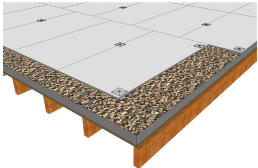
Figure 1: Underlayment Fastener Suggested Pattern
